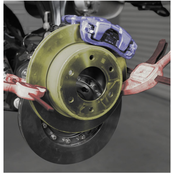
W/O Tool Rear Flip Supplied Rear Rotor Inside Out Clamp Factory Rotor to Supplied Rotor Place caliper on Rotor Rotate Upward to Factory Position
