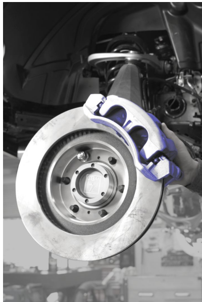
W/O Tool Front Flip Rotor Inside Out Place caliper on Rotor Rotate Upward to Factory Position
