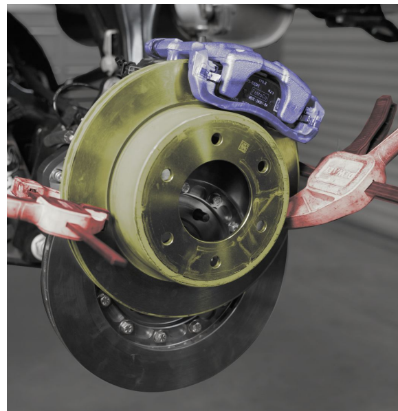
W/O Tool Rear Flip Supplied Rear Rotor Inside Out Clamp Factory Rotor to Supplied Rotor Place caliper on Rotor Rotate Upward to Factory Position
